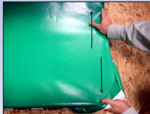
Figure 8 Before tensioning with the Tension Tool, push and pull the material to eliminate some of the pucker.
