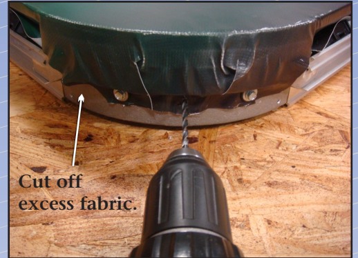
Figure 15 Cut excess fabric off by following the groove underneath the fabric on the cast Radius Corner where it recesses to a lower level. Pre-drill holes for security screws just below where the tape is located.
