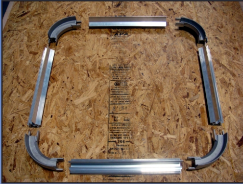
Figure 1 Lay out extrusion lengths and cast corners.
