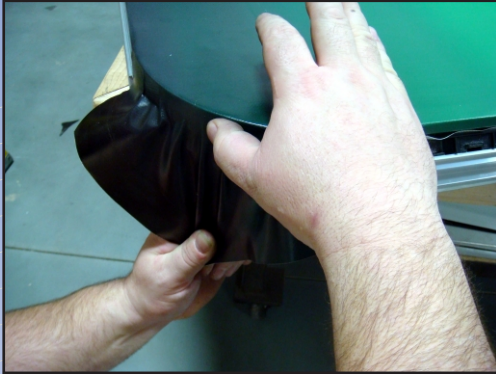
Figure 13 Work the flexible fabric to eliminate puckering or wrinkles while pushing it onto the tape.
