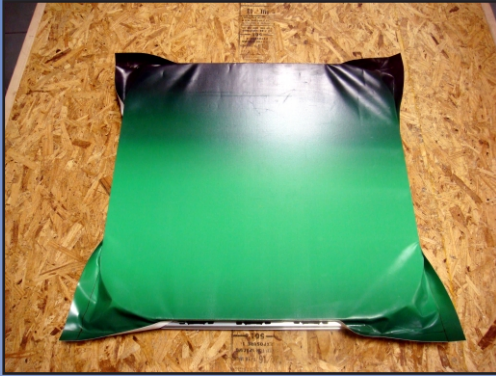
Figure 10 Once the straight areas of fabric are tensioned flat, do not continue to push the clips in farther. The corners may still have puckering.
