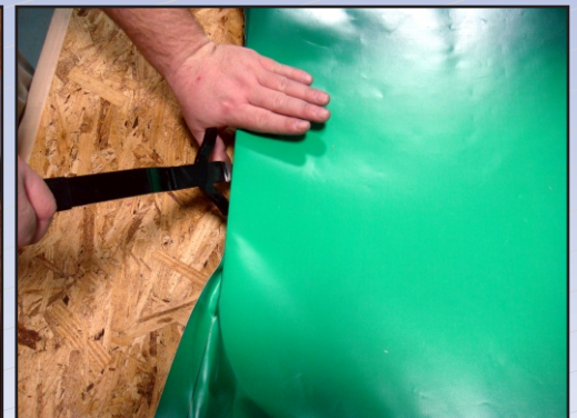
Figure 9 Using the Tension Tool, start working around the frame pushing the Tension Clips in one click at a time. You may find it helpful to continue to push and pull the fabric in certain areas.
